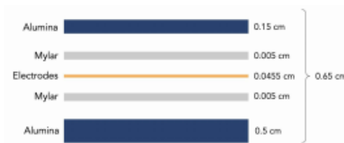
Fig. 5 Exploded view of layered panels. Figure not to scale.
